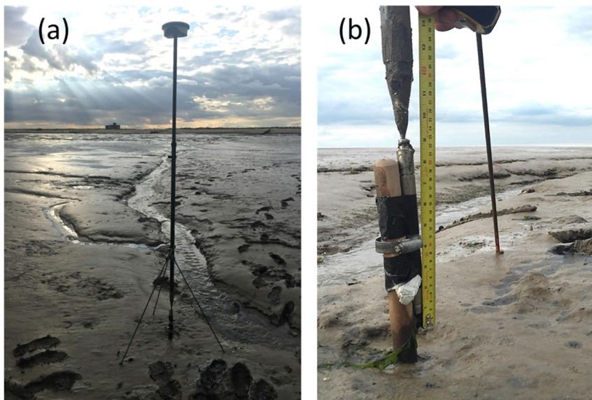
Figure 167: Measuring the location of PS2 at Shell Ness on 29 July, 2015: (a) Leica station positioned above PS2; (b) close up of position measurement.
